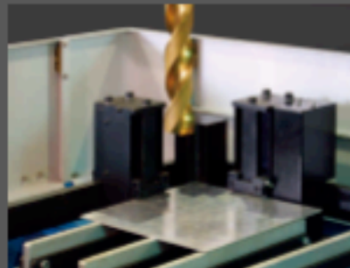
Supporting block, hydraulic dampers, Automatic plate thickness measuring device
